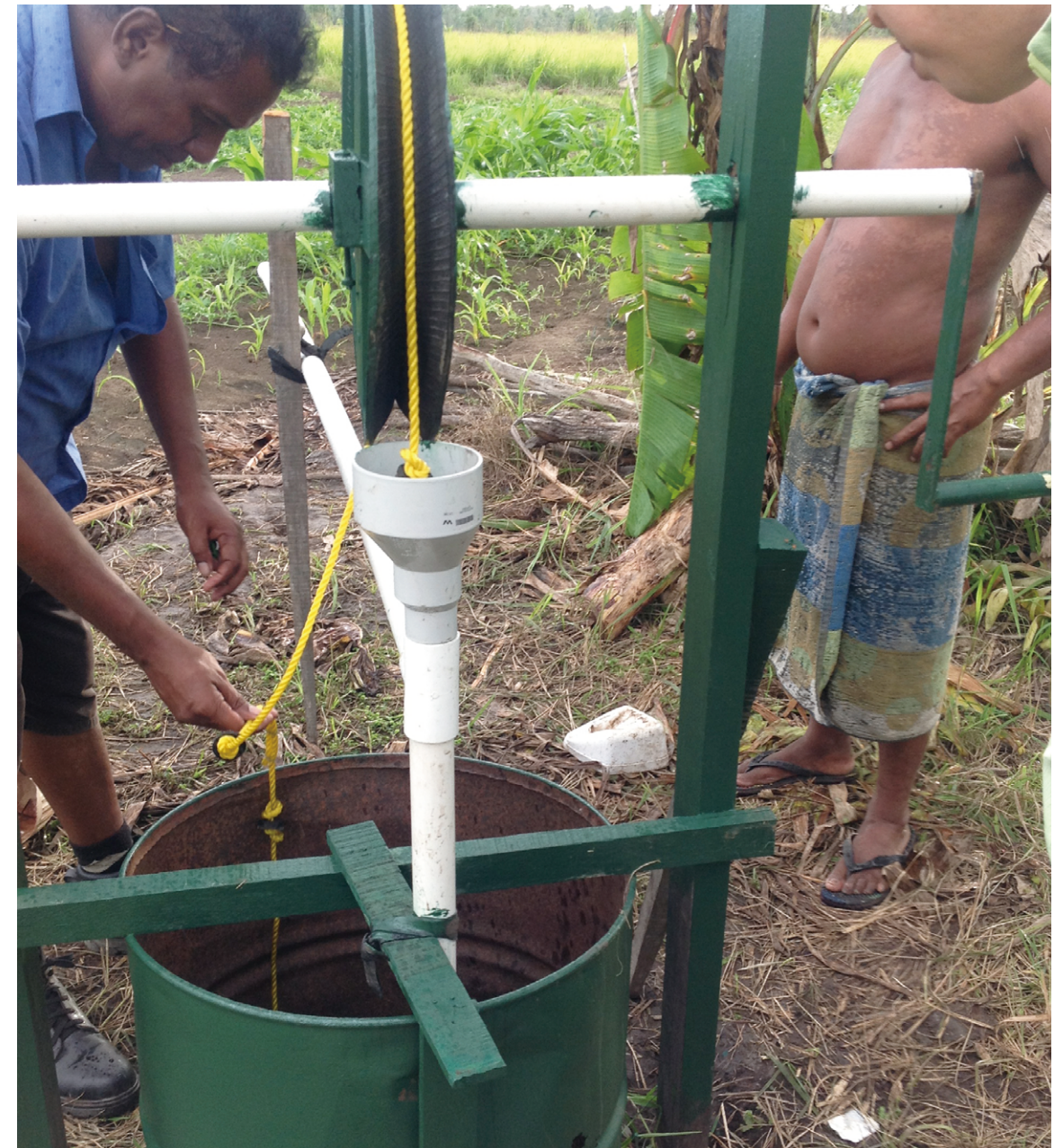
This is a picture of the kind of water pump initially in use. By turning the green handle, you spin the pulley, causing the yellow rope with the black washers (the discs between each knot) to draw the water up through the pipe.
