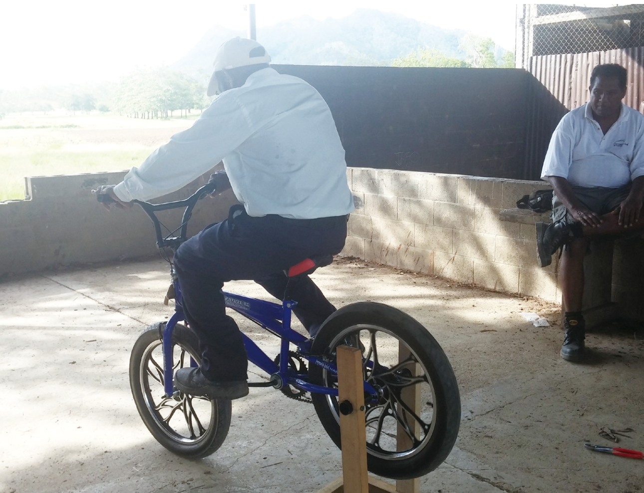
The new bicycle-operated pump is being tested. Since it requires only one-eighth of the labor necessary for turning the handle of the previous model, the irrigation process is made much easier.
