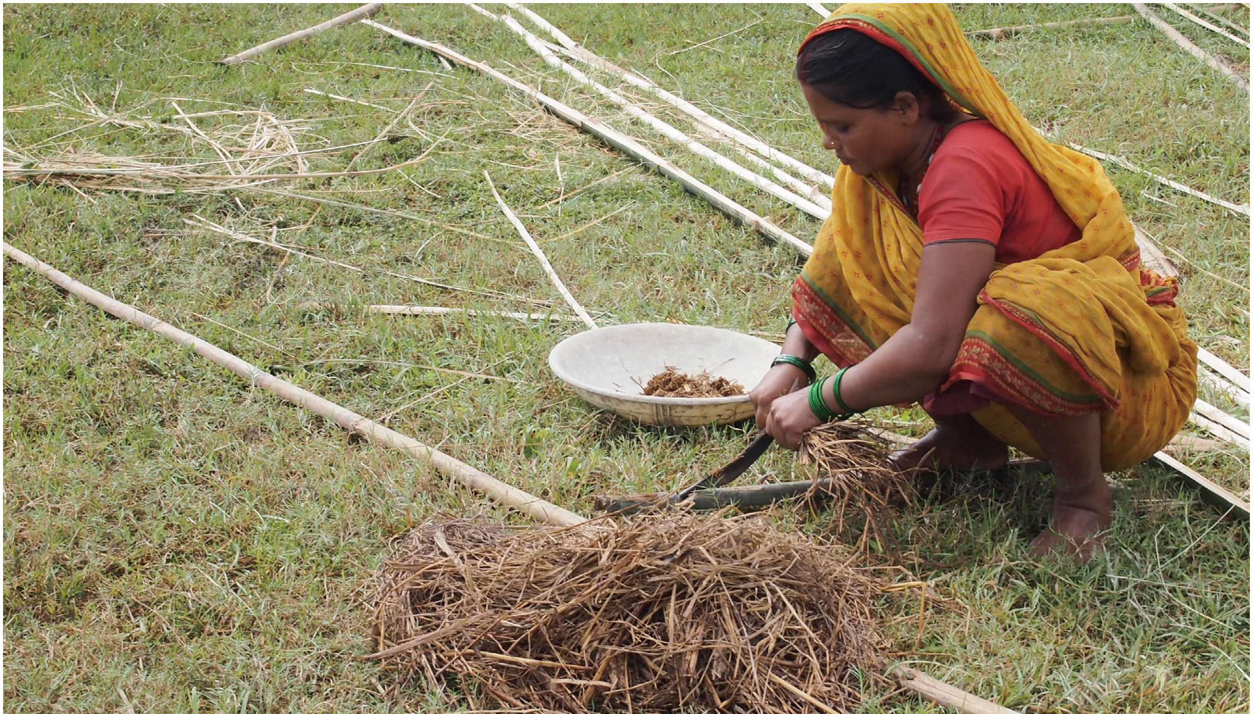
An experiment with a mixture of local mud and straws to replace cement in making wall surfaces more durable.
